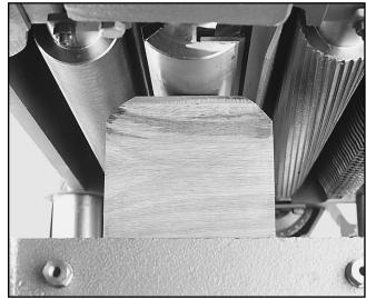
Figure 11. Guide block indicates parallelism.
